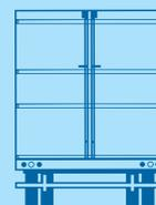
The bonded foam "sandwich" design improves thermal performance and seals better than any other design. External "hat" sections mount all door hardware without "thru-holes" into the internal foam cavity, reducing moisture entry points, keeping the foam dry, and optimizing thermal performance.
